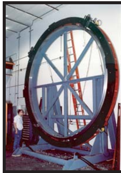
World's largest gear driven clamshell lathe on giant mock-up at D.L. Ricci's Red Wing HQ
